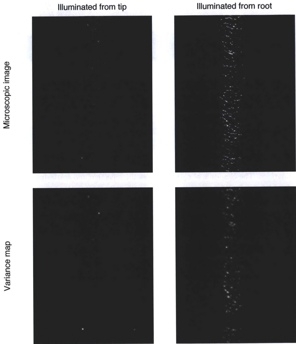
Figure 3-5: Images of healthy black hair captured by the prototype and their processed images. The top row shows the original microscopic images. The bottom row shows their local variance map. Illumination from root side enhances the contrast at the edge of cuticles.
