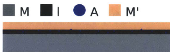
Figure 1.1: conventional metal-insulator-metal IETS Devices
