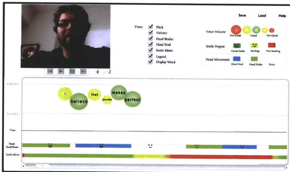
Figure 5-3. Iteration 3 of the interface. A video of the participant is added to the interface. The smile meter now contains smiley faces.
