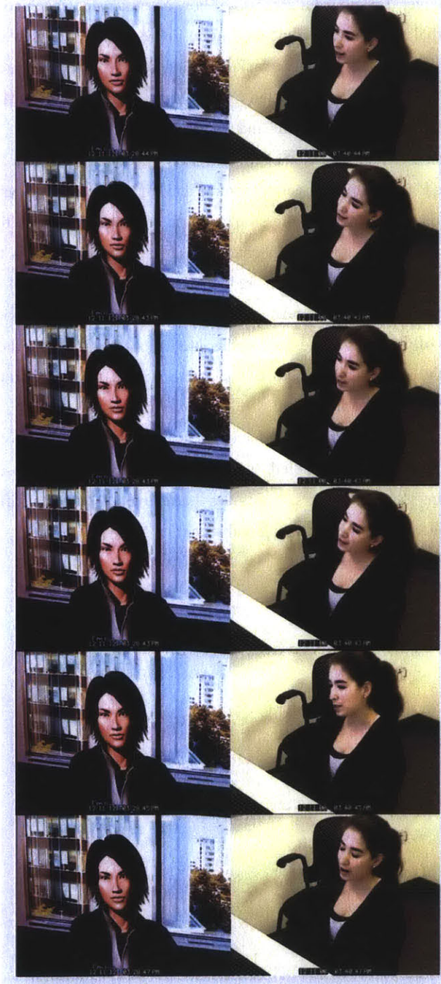
Figure 6-9. The virtual agent is mirroring the head tilt of the participant in real-time. This figure displays successive frames of a video, showing the progression of the mirroring.
