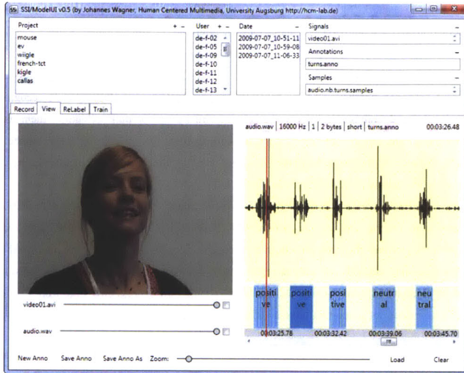
Figure 2-4. SSI GUI that allows developers to record training data and build user-dependent or user-independent models out of it. The screen shot provides a snapshot of a session with video and audio data (J. Wagner, Lingensfelder, & Andre, 2011)
