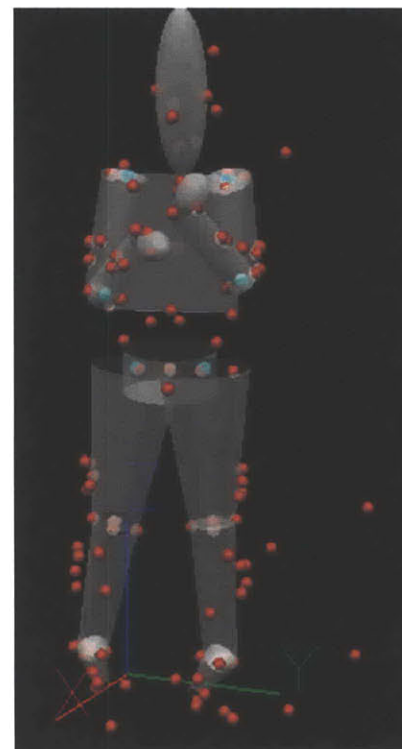
FIGURE 2-8 Inferring the skin surface location from marker position allows for segment definition.
