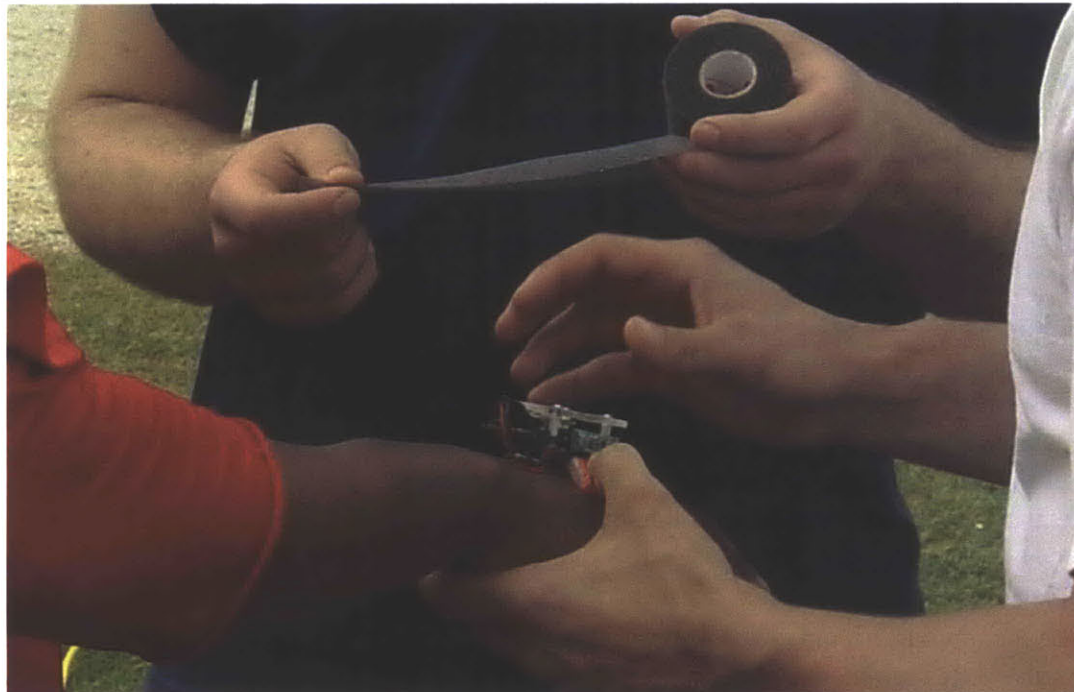
FIGURE 7-59 Node mated to hand with stim pad and about to be pre-wrapped.
