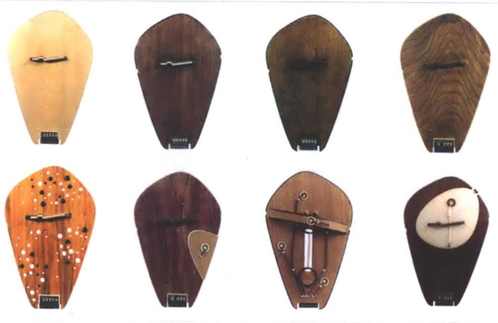
Figure 3.11: Figure 10. Top: A group of eight resonators. The first four are more traditional, made from wood only. The last five are more experimental, including loose screws, springs, free plates or plastic chamber with rice or water. Resonator no. 1 (top left) was used as the reference for algorithm development.
