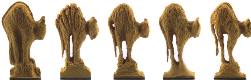
Figure 2.20 Five cats made by five participants using the FreeD, all using the same CAD model.
