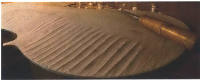
Figure 2.32 Marco's violin-making process, carving traces with gauges in the rough stage of the work.
