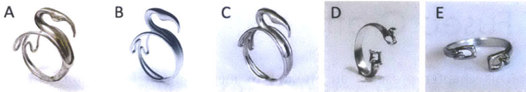
Figure 4.1: The original, hand-made swan ring made of silver (A), CAD model of the ring (B), and the 3D printed silver replica (C); the hand-made miniature hands ring (D), and its replica (E).
