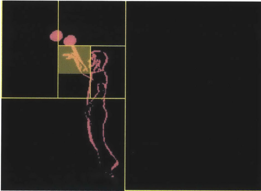
Figure 5-1: A mock-up of the divide and conquer approach that can be used to optimize image processing and finding the best attentional locus. The pink pixels are the non-zero locations of the frame subtraction operation.
