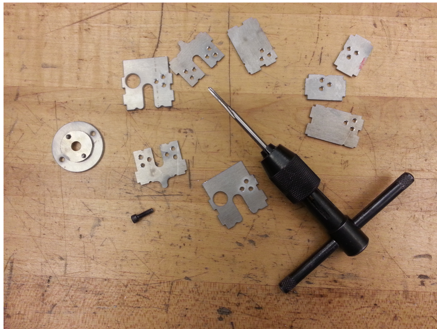
Figure 3-2: Some Components Require Holes to be Threaded with a 4-40 Tap
