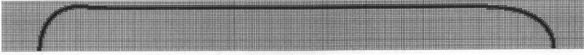
Figure 4-8: Typical computational mesh used for slug flow simulations. Shown is the mesh for Ca = 0.05 .
