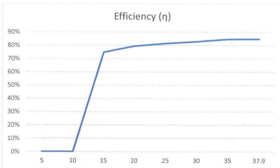
Figure 49: Converter Efficiency with D=0.5 and Variable Input Voltage
