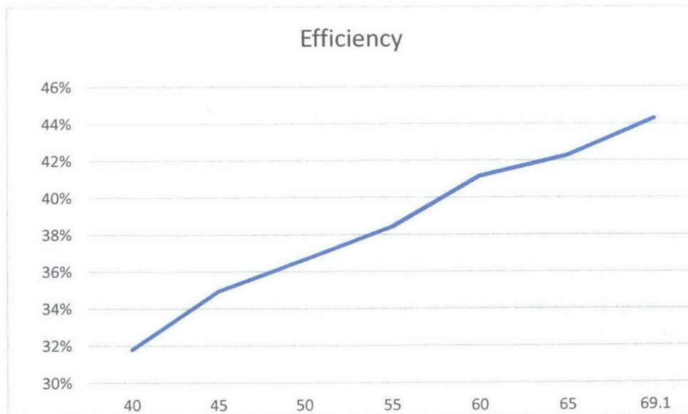
Figure 50: Converter Efficiency with D=0.1 and Variable Input Voltage
