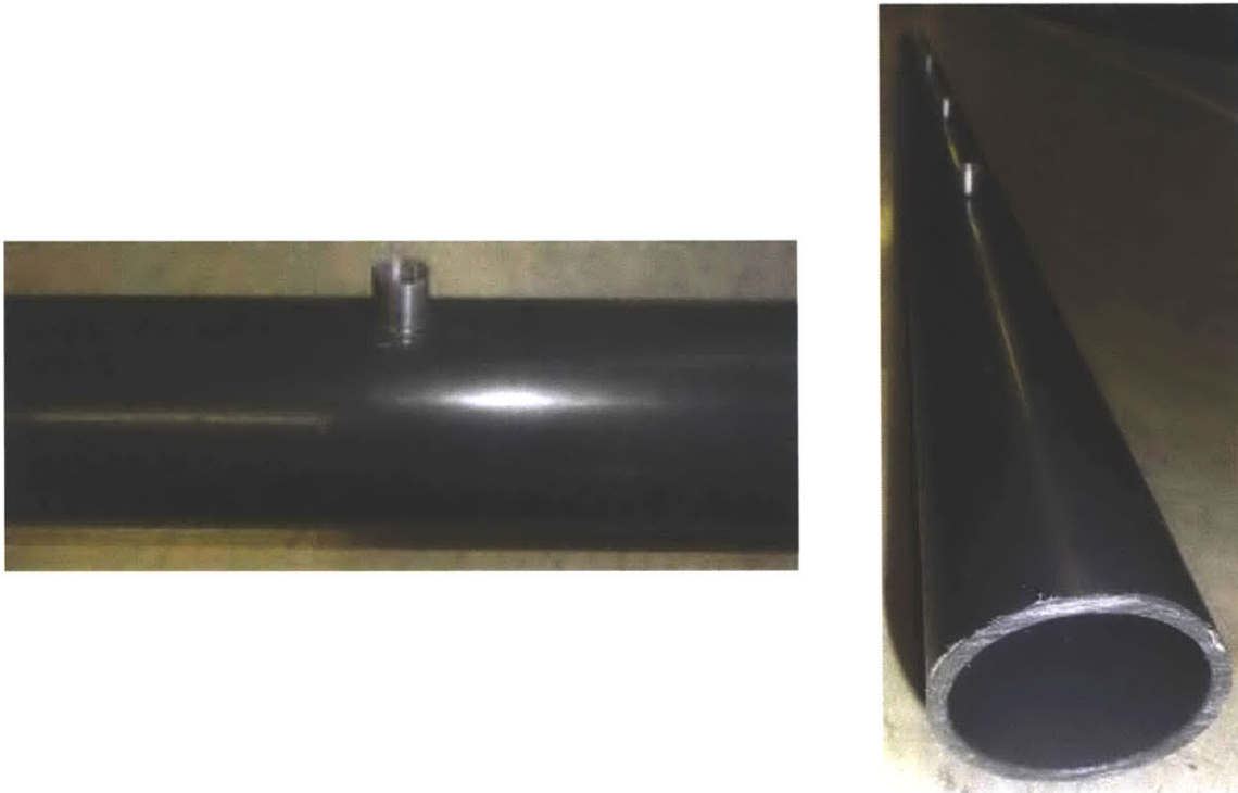
Figure 22: Microphones are stationed along a pipe to measure entropy noise in the test rig. Microphones are flush mounted so they do not disturb airflow.
