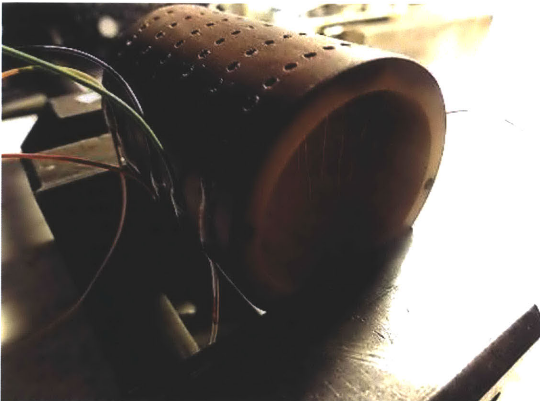
Figure 13: The entropy wave generator (EWG) heats electrically. Platinum-rhodium wires are strung through holes piercing through a housing tube like thread through a button.
