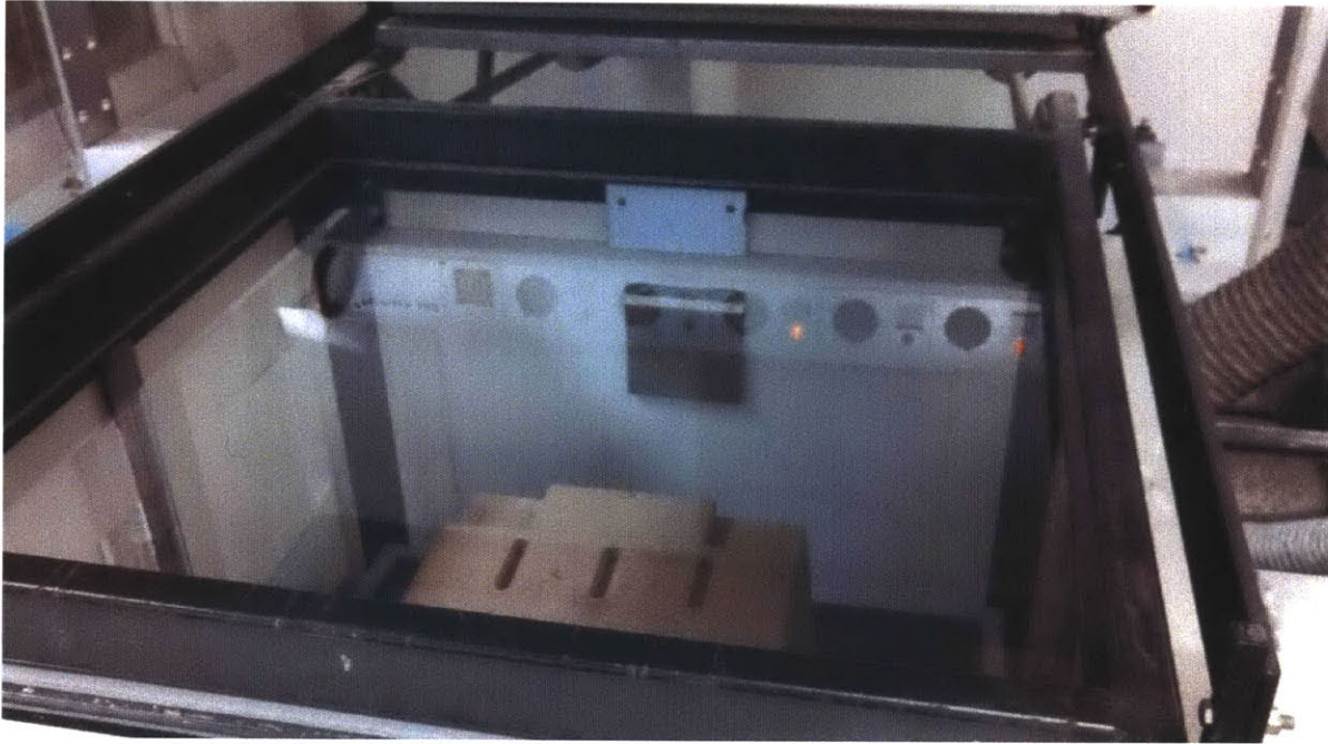
Figure 3-3: Setting-up the body mold in the thermoformer
