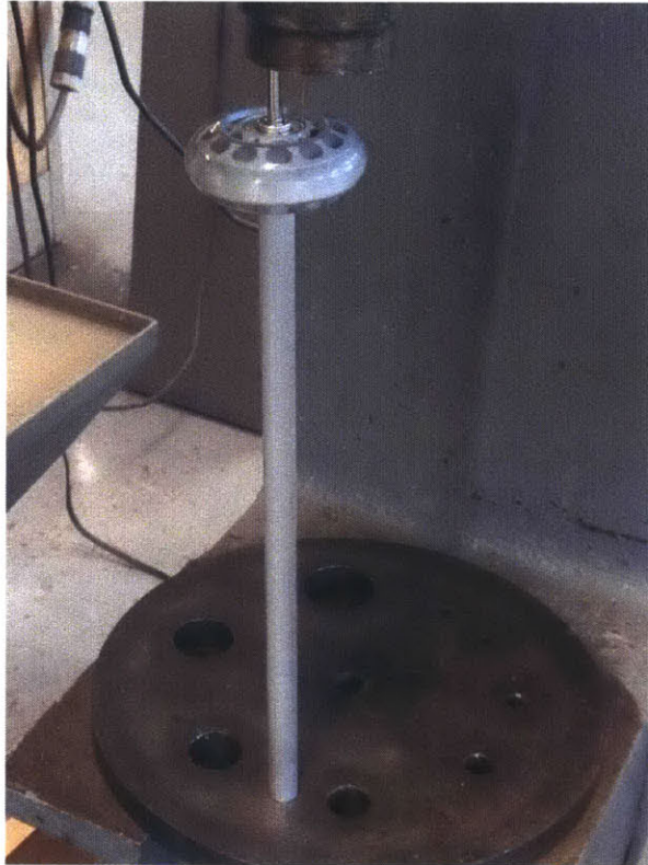
Figure 4-15: Using the arbor press to insert the pins into the axle.
