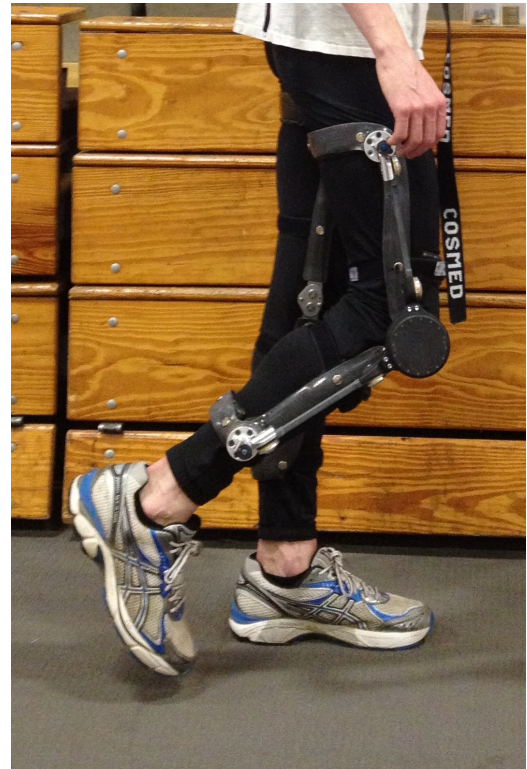
Fig. 3. Clutch-spring knee exoskeleton, as worn here. Figure from [17].
