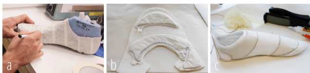
Figure 12. Fabrication process of Jamming Shoes
