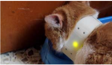
Figure 7. TagMe detects when a pet is eating and sends a notification to the owner.
