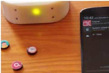
Figure 3. Feedback provided after detecting a tag: LED and smartphone popup.
