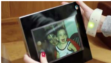
Figure 8. The user is touching her picture and the system is sending a notification to her contact.
