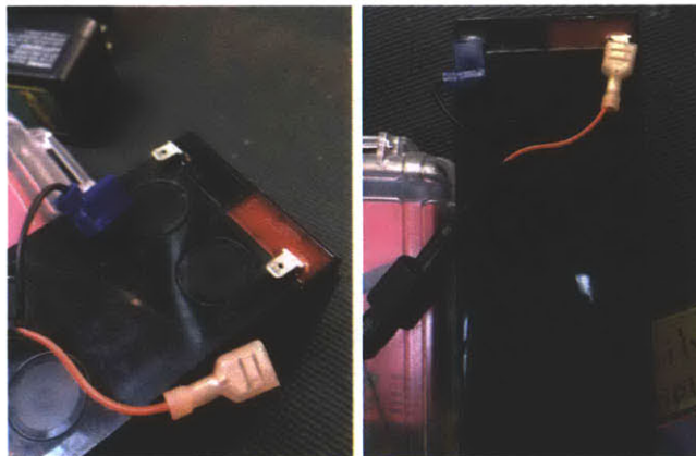
Figure 9: Battery connectors are attached to end of power pigtail cable. These connectors fit over the battery terminals to power the payload computer module.
