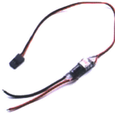
Figure 7: A universal battery elimination circuit. The bare wires take an input voltage between 5 and 23 volts, and the circuit outputs 5V at 3A.
