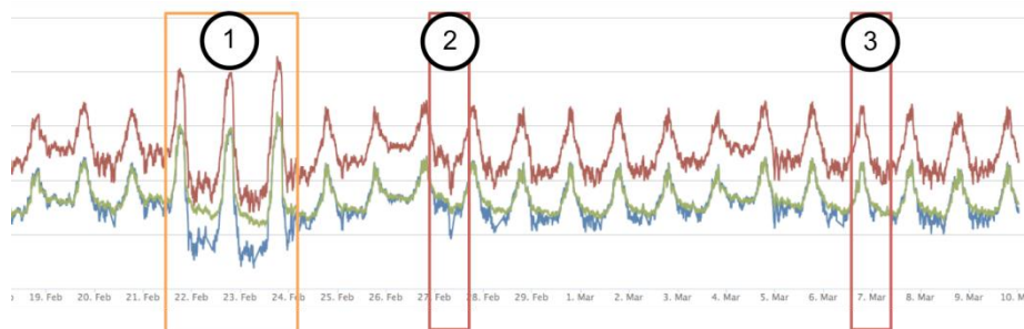
Figure 7: An example of an event post-mortem, where (1) shows an unusual operation, (2) shows a suspected break event and (3) shows the first reports of leakage. Pressure is shown in meters.
