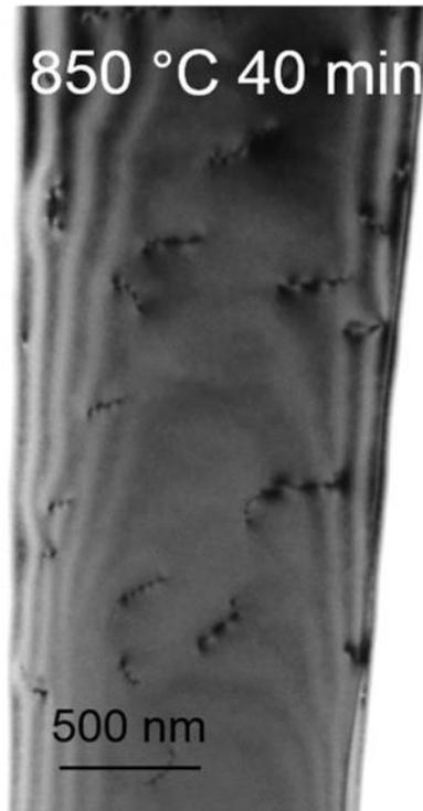
**Figure 4.13** Plan-view TEM showing uniform threading dislocations in a 1 μm wide and 350 nm thick n-type Ge waveguide by annealing at 850 °C for 40 min. (TEM courtesy of Tim Milakovich)
