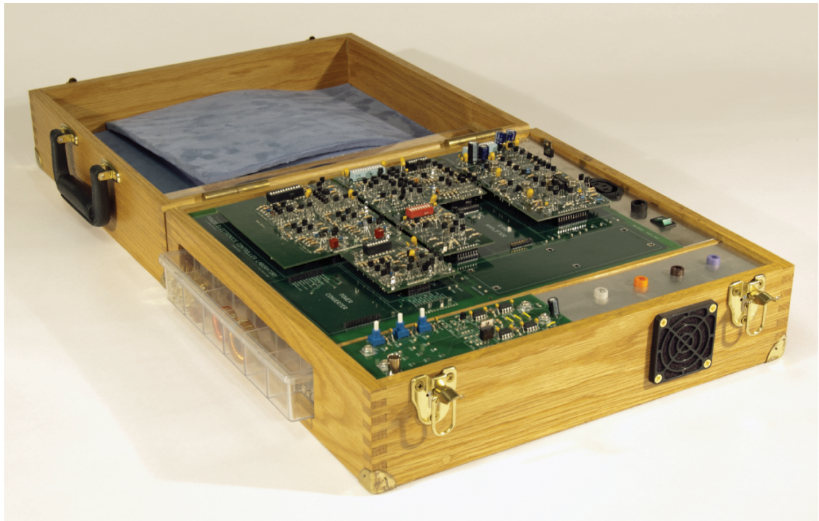
Figure 6-2: An overall view of the power electronic controller kit. The wooden box houses the motherboard, on which the various controller circuit blocks are mounted. The box also has a place for storing the kit components (courtesy of Mark Avestruz, 2012).
