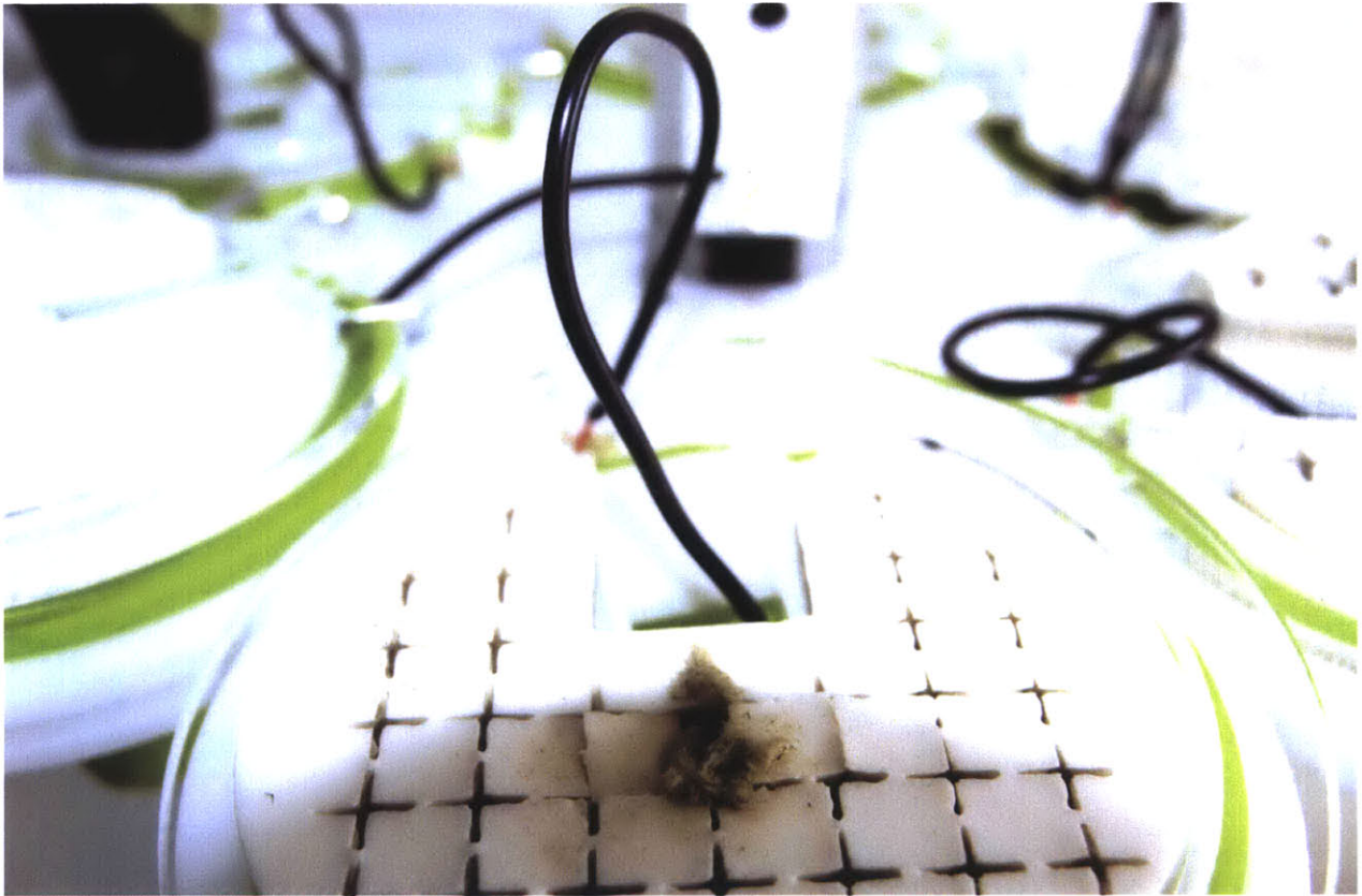
Figure 8.3 Problematic wiring of misters through center of sleeves, this may be addressed through the insertion of the sensor circuit board. Also note that not all sleeves are secured within the pod.
