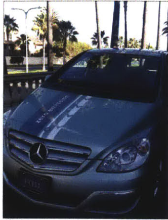
Figure 1.1. Mercedes-Benz B-Class F-CELL hydrogen fuel cell electric vehicle. These cars have been in operation in Europe and the US since 2010, and similar versions will be available to consumers in CA in 2015.
