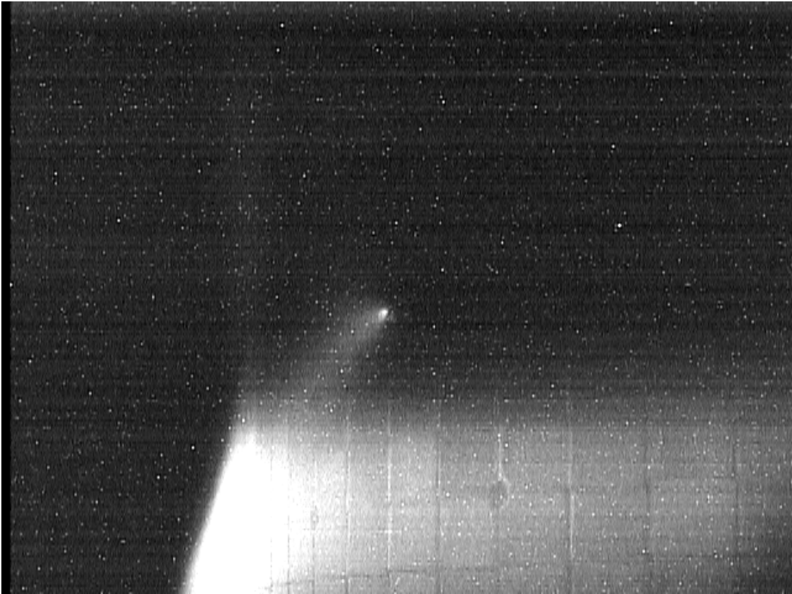
Figure 5-2: Recorded image of the inner wall showing the plume from a gas puff with the MARFE below the gas puff and the plume tail pointing towards the MARFE.
