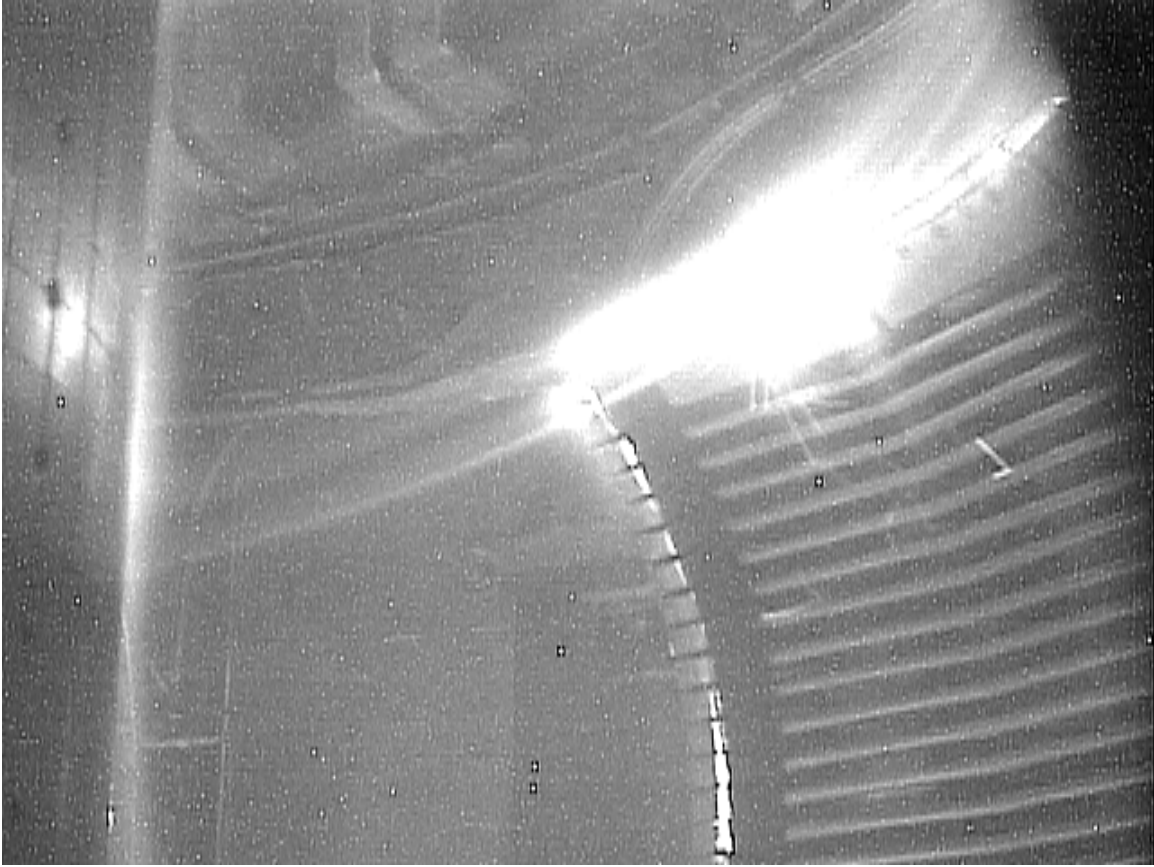
Figure 3-1: Sample camera image showing “sparks” coming from the RF heating antenna structure.
