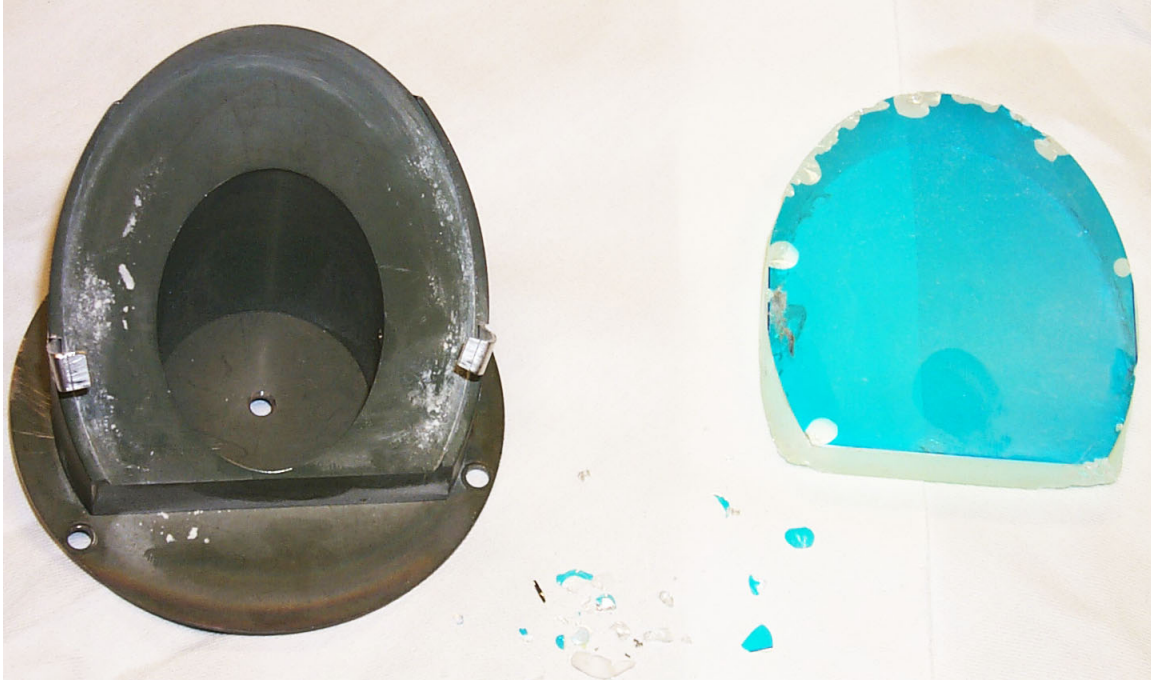
Figure 3-6: Early MSE mirror mounts had many metal to glass interfaces. Every instance of metal to glass contact resulted in damaged optics, like this early M1, which rested on a steel base, held by metal tabs. Damage occurred on both front and back surfaces of the mirror.
