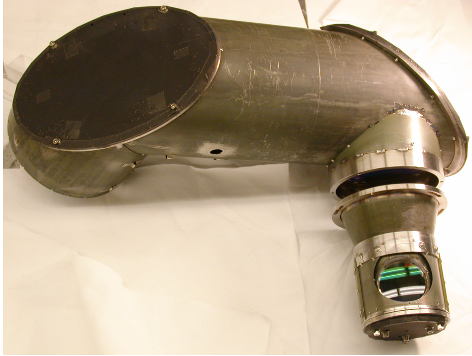
Figure 3-15: Modified MSE split can allowing viewing angle adjustment and removal through a reentrant port.
