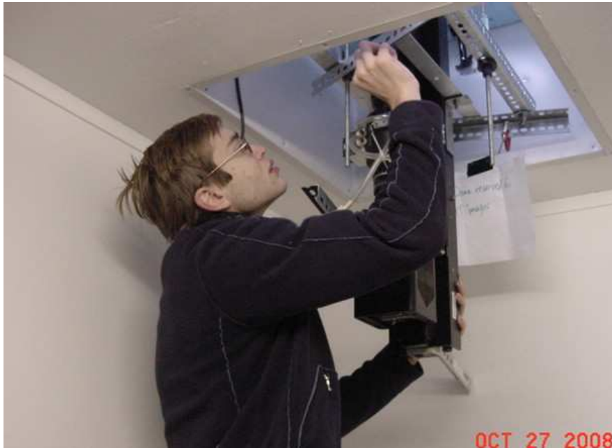
Figure 2-1: Mounting All Sky Imaging System (ASIS) in HAARP Optical Shelter for experiments
