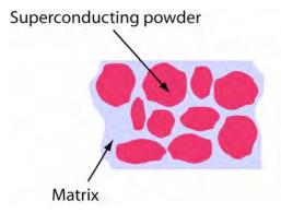
Fig. 15. Schematic diagram of hyperconducting material
