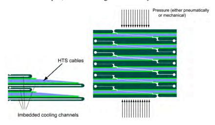
Figure 11 (a) Schematic diagram of the joint region in a section of a toroidal field segment; (b) Illustrative design of joint during operation, with pressure applied for current transfer between cables in different section of the TF coils
