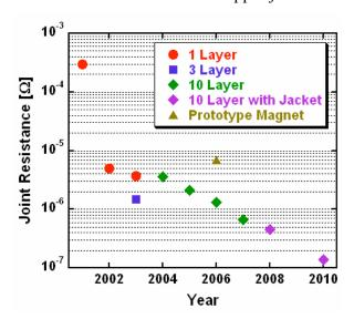
Fig. 8. Progress in performance of butt joint.
