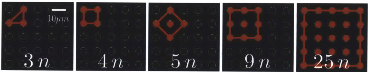
Figure 3-6: Representation of measured area with the n point technique: the n point averaging techniques corresponds to a moving best square fit of the deformation gradient tensor \overline{\overline{F}} describing the deformation of the microscopic are defined by the n markers
