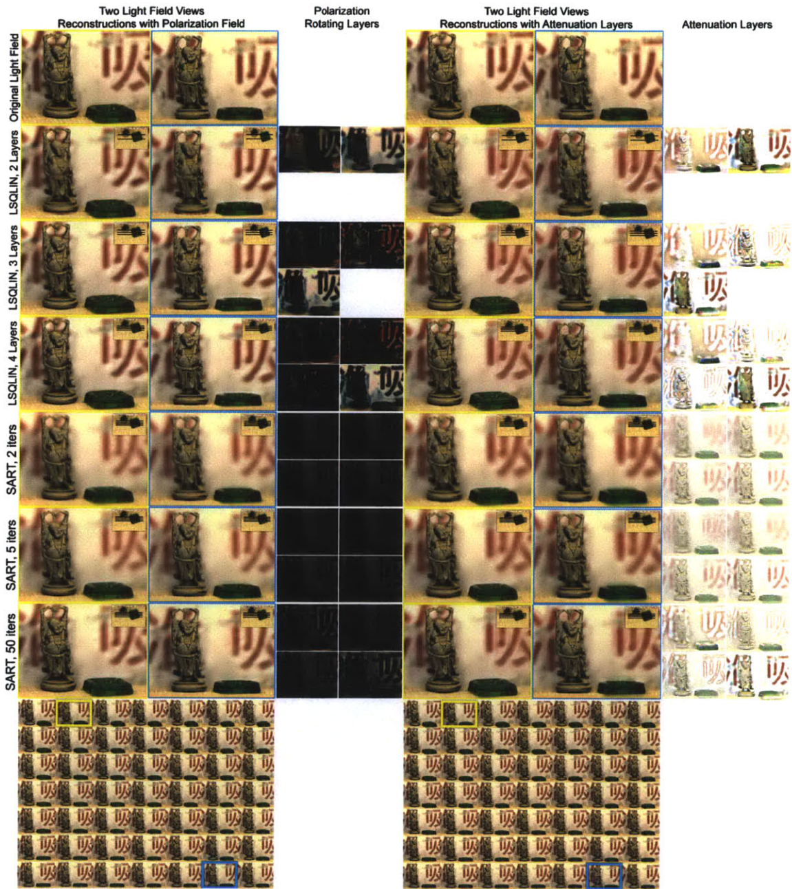
Figure 3-12: “Buddha” scene, using the “Buddha” model from http://graphics.stanford.edu/data/3Dscanrep/ . Simulated views are compared for polarization-rotating layers (first and second columns) and attenuating layers (fourth and fifth columns). Rows illustrate, from top to bottom: target views, reconstructions using the off-line solver for two, three, and four layers (for the same depth range), and SART reconstructions with two, five, and fifty iterations with four layers. Columns three and six present decomposed layers.
