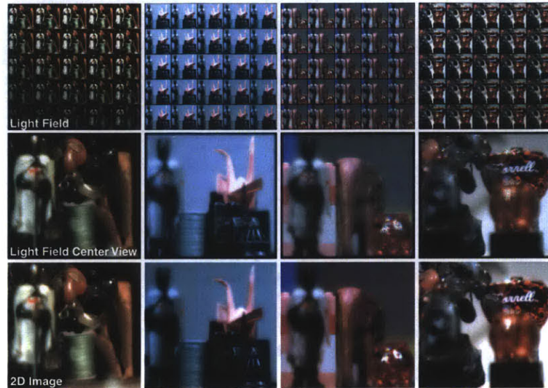
Figure 4-9: Overview of captured scenes showing mosaics of light fields reconstructed via sparsity-constrained optimization (top), a single view of these light fields (center), and corresponding 2D images (bottom). These scenes exhibit a variety of effects, including occlusion, refraction, specularly, and translucency. The resolution of each of the 25 light field views is similar to that of the conventional 2D images.
