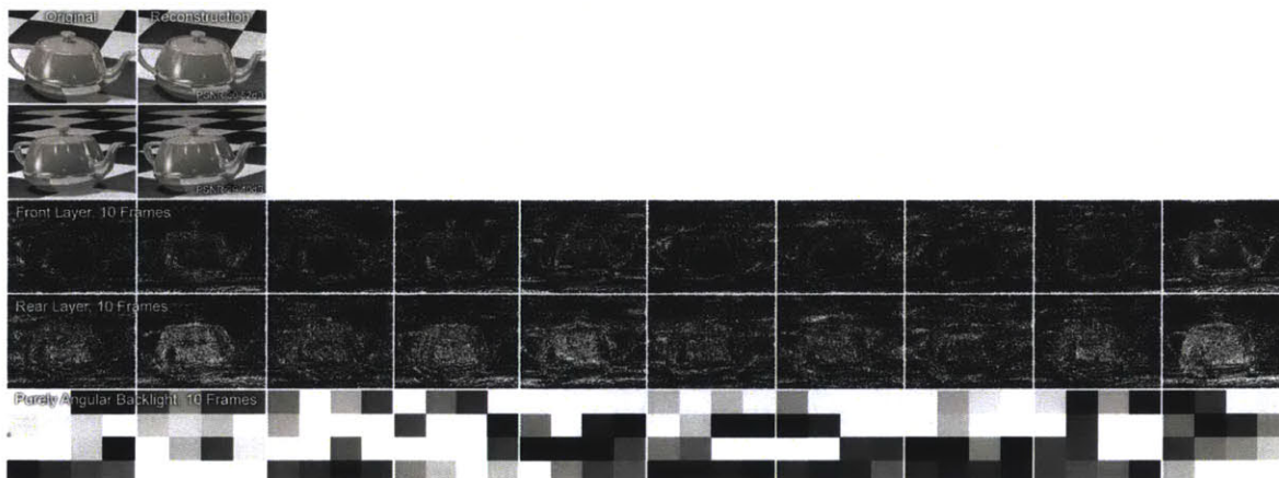
Figure 3-51: Decomposition for dual-layer display containing a purely angular backlight behind the rear layer. The original light field has 4 \times 4 views within a field of view of 30^\circ . Two of the original views are shown on the upper left with corresponding reconstructions next to them. This data set represents a rank-16 light field, which is decomposed using 10 frames. The two layers are separated by a distance that corresponds to the separation distance for an equivalent parallax barrier display. Each frame is shown for the front layer (row 3), for the rear layer (row 4), and for the angular backlight (bottom row). The layer decompositions resemble what NMF produces for dual-layer setups (see Section 3.3), but adds an angular backlight (see Section 3.4.7) for improved depth of field and field of view.
