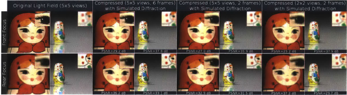
Figure 6-9: Simulated retinal blur and diffraction. Images show closeups of close and far matryoshka dolls from the light field shown in Figure 6-2, and inset images show further magnification. The larger doll is virtually positioned at 17 cm in front of the display and the rear doll at 18 cm into the display. The views of the light field are evenly spaced over a pupil of a = 5 mm for a single eye, with the outermost views centered at the pupil edges. Compressed images reflect the configuration of our prototype display: 1 LCD layer in front of a HARB, a f = 31.8 cm focal length lens, a viewing distance of d_e = 127 cm, and native panel resolution of 39.1 cycles/degree at this distance. Diffraction is approximated using the method described in Section 6.1.1 using the wavelengths \lambda_{red} = 700 nm, \lambda_{green} = 546 nm and \lambda_{blue} = 435 nm. Rows: Synthetically refocused images of front doll ( first rows ) and rear doll ( second rows ). First column: Source light field. Following three columns: Compressed version of the source light field using the decomposition algorithm described in Section 6.1.1 in the noted configurations. High quality retinal blur can be achieved in the presence of diffraction ( second column ), but quality suffers if compression is too high ( third column ) or angular resolution is too low ( fourth column ).
