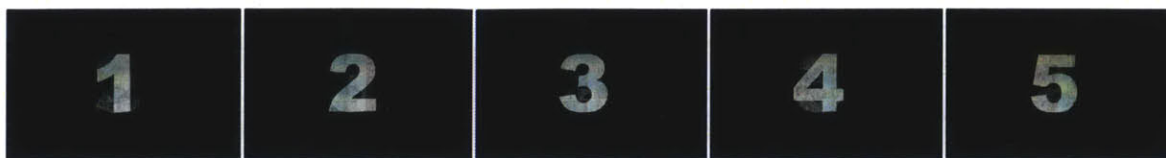
Figure 3-50: Synthesis of uncorrelated views. Five photographs of the three-layer prototype showing the performance of a rank 12 factorization for a light field comprising uncorrelated views (i.e., Arabic numerals in this example).
