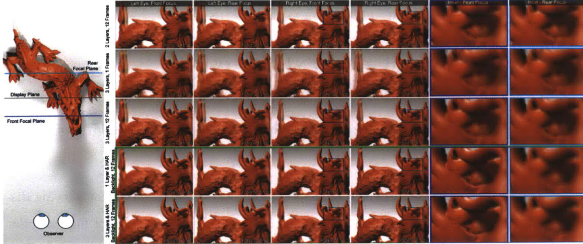
Figure 6-4: Performance of computational displays vs. display complexity. We simulate the ability to refocus the light field emitted from various displays, with and without HAR backlighting, following the design proposed in Section 6.1.1. Up to three layers were placed in front of a Fresnel lens, with focal length f = 30 cm, each separated by 0.5 cm. We decompose the target light field to emit 5 \times 5 views spanning each viewer pupil, separated by a distance d_e = 100 cm from the lens. Left: The light field corresponding to a dragon model is provided as input to the decomposition algorithm. Right: The first four columns show the received images for the left and right eye, when focused in front of and behind the lens. The remaining two columns show inset regions centered on the dragon’s eye. Five system architectures are compared from top to bottom, with varying numbers of layers and frames. The first three rows evaluate Tensor Display designs using a uniform backlight ( b_m(x, v) = 1 ). The last two rows illustrate the benefits of HAR backlighting, demonstrating that its inclusion enables clear focus cues; note that the dragon’s eye can be brought into sharp focus, in contrast to cases without HAR backlighting. Quantitative assessment of focus is provided by the peak signal-to-noise ratio (PSNR) with reference to the original refocused light field, confirming that increasing layers and frames reduces artifacts.
