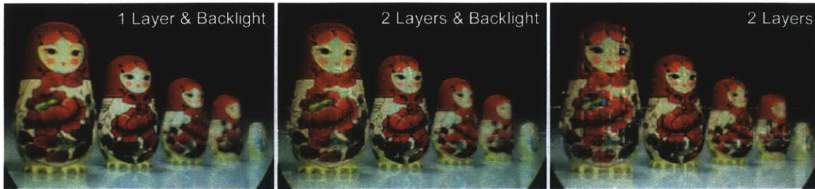
Figure 6-13: Failure case photographs for dual layer architectures. In practice imprecise alignment of prototype layers creates artifacts. Artifacts are also observed in simulation, as narrow view spacing poses a challenge for large LCD pixel sizes.
