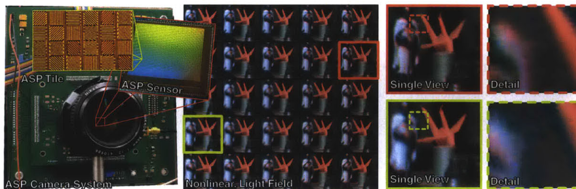
Figure 4-1: Prototype angle sensitive pixel camera (left). The data recorded by the camera prototype can be processed to recover a high-resolution 4D light field (center). As seen in the close-ups on the right, parallax is recovered from a single camera image.
