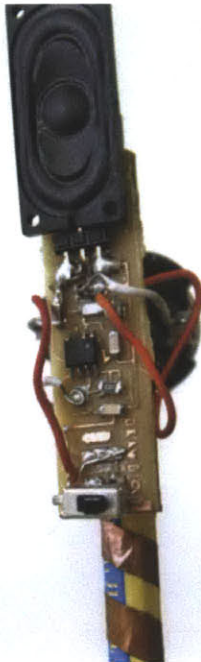
Figure 5.24. Mechanical pencil with Modela-milled Drawdio circuit attached. The mechanical pencil had the attachment to the metal tip of the pencil which came into contact with the graphite as opposed to the screw into the top of the pencil.
