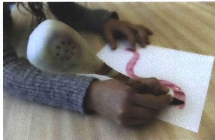
Figure 5.26. Left: a musical jacket with the Drawdio circuit inside "Ok2Touch". Right: a musical paintbrush with the Drawdio circuit inside exhibited in museums
