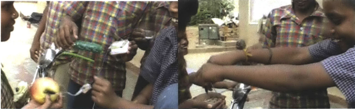
Figure 5.10. Left. Listening to the sound of the resistance of an apple with a PicoCricket. Right. PicoCricket resistance-to-sound measuring dirt.
