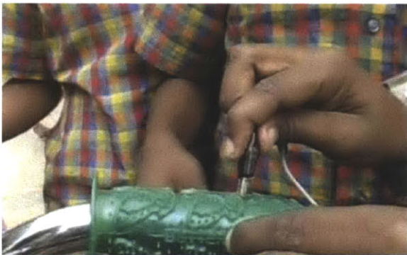
Figure 5.11. Pico Cricket resistance-to-sound measuring rubber or plastic bicycle grip
