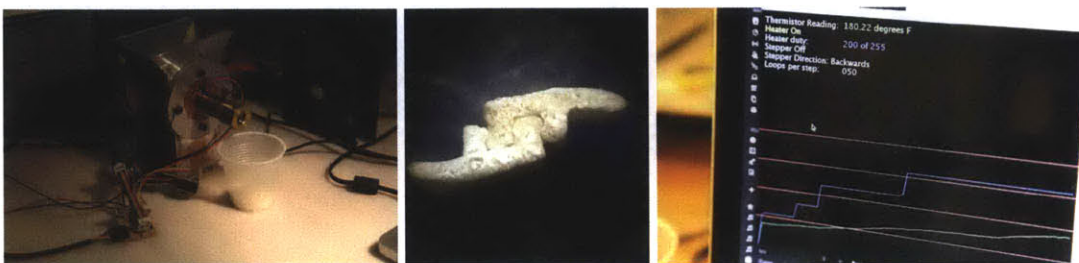
Figure 7.6: A) Ziploc extrusion machine, B) Microscope photograph of interlocking ziploc elements (roughly 6mm across), C) Graphical user interface for the extruder.
