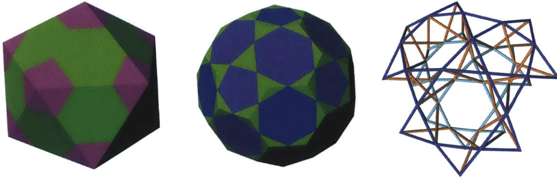
Figure 7.2: Constructing the spherical lattice by truncation of polyhedra.
