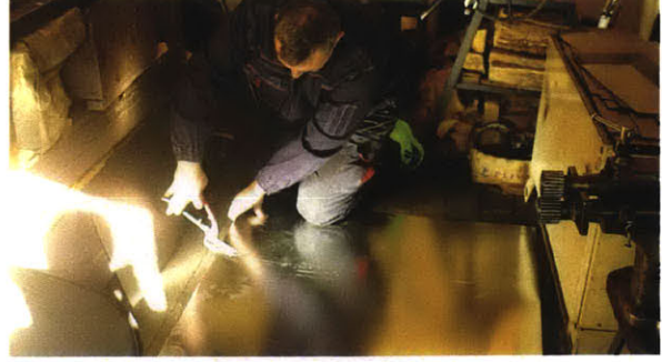
Cutting the sheet along the mark made previously
