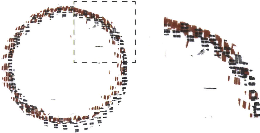
Figure 3-6: Scan of a print showing alternate white and dark bands because of the onboard FTDI buffers. Contrast this with figure 3-9 which was printed by tuning the USB FTDI buffers as described in section 3.4.2.
