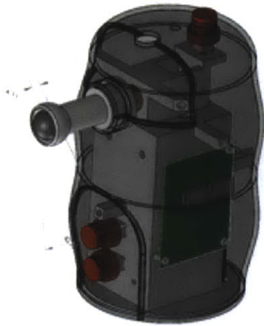
Figure 3-18: The solidworks CAD model of the handset showing internal chassis that mounts the circuit boards, buttons, tracking sensor, digitizer and printhead.
