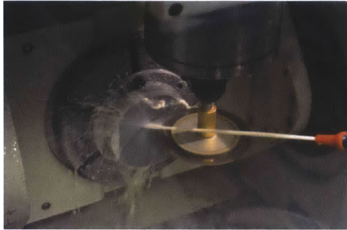
Figure 2-13: Dicing a silicon wafer in the Hurco VM10U.
