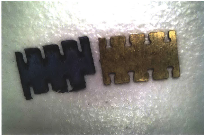
Figure 2-12: Excimer cut part next to brass part produced using the Wire-EDM.
