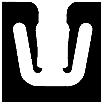
Figure 2-4: Potential scraping/wiping contact slot design.
