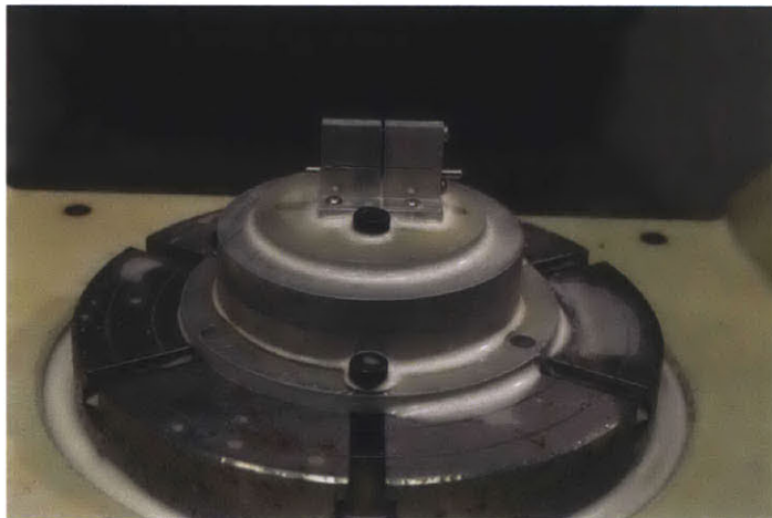
Figure 2-16: Fixture used to cut slots in the parts
