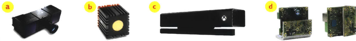
Figure 2-5: Consumer and industrial grade ToF cameras. (a) PMD CamCube (photonics mixer device) (b) Mesa (also known as the Swiss Ranger) (c) Microsoft Kinect (d) PMD Nano.
