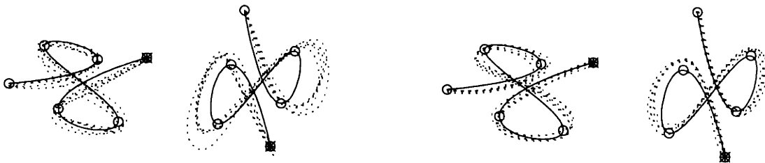
Figure 6-5: Examples of paths traced in task 3. Each pair of plots is data from one subject (six different subjects shown). The solid line is the minimum jerk path (which was not shown to the subjects), and the dotted lines are the actual paths on the last 5 trials of the 10 trial block. The filled circle marks the end point.
