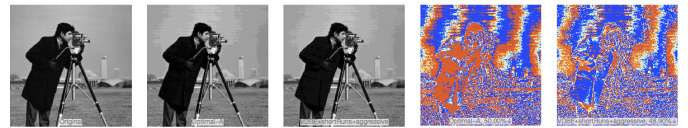
(d) From left to right: Original image, e_4(s, m) encoded, Rake encoded, e_4(s, m) image difference, Rake image difference.
