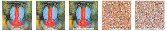
(c) From left to right: Original image, e_4(s, m) encoded, Rake encoded, e_4(s, m) image difference, Rake image difference.
