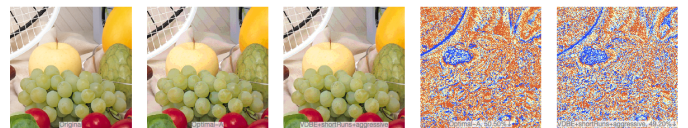
(f) From left to right: Original image, e_4(s, m) encoded, Rake encoded, e_4(s, m) image difference, Rake image difference.
