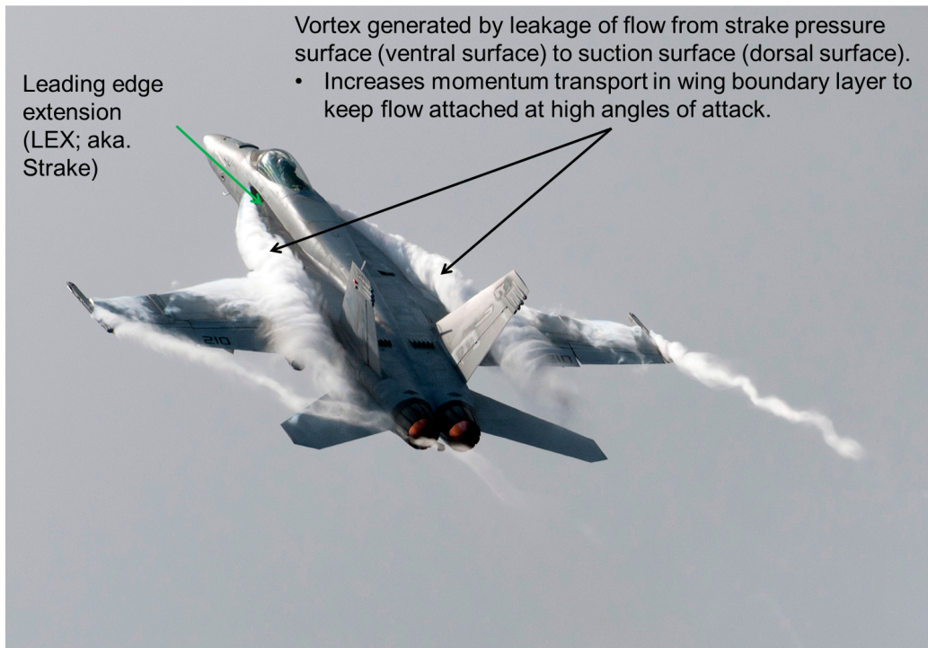
Figure 4-31: Operational example of leading edge extension (i.e. strake) on a F-18 Super Hornet used to generate a vortex along wing upper surface to delay separation. Source: Wikipedia, http://en.wikipedia.org/wiki/Strake_(aeronautics)
