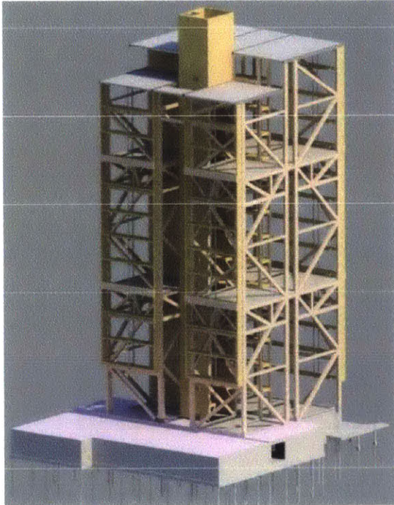
Figure 23 - Treet Structural System
