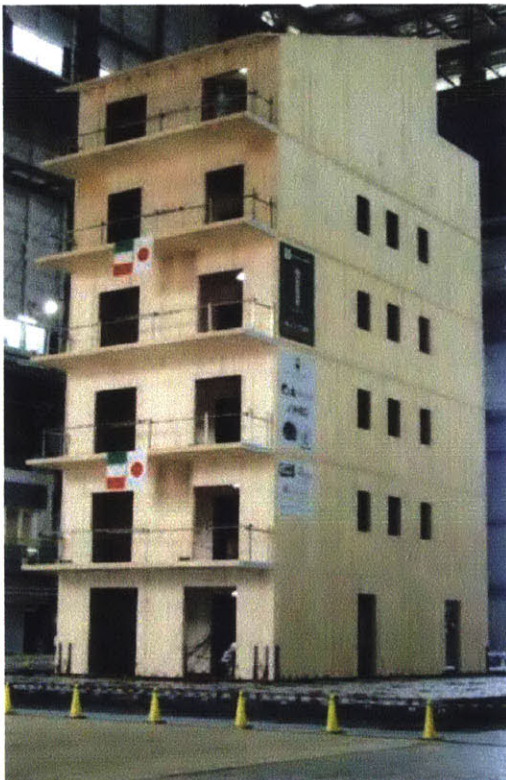
Figure 29 - CLT Building on Shaking Platform (Japan)
