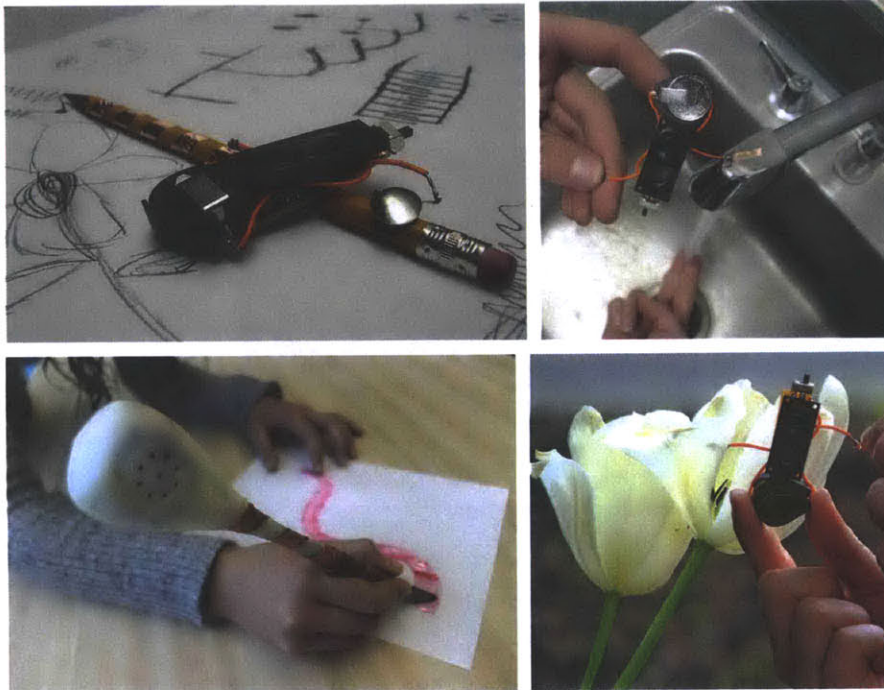
Figure 6: Drawdio inventions that make music by measuring the resistance of, clockwise from top left: a graphite pencil drawing, a stream of water from a faucet, a flower, and a watercolor painting.
