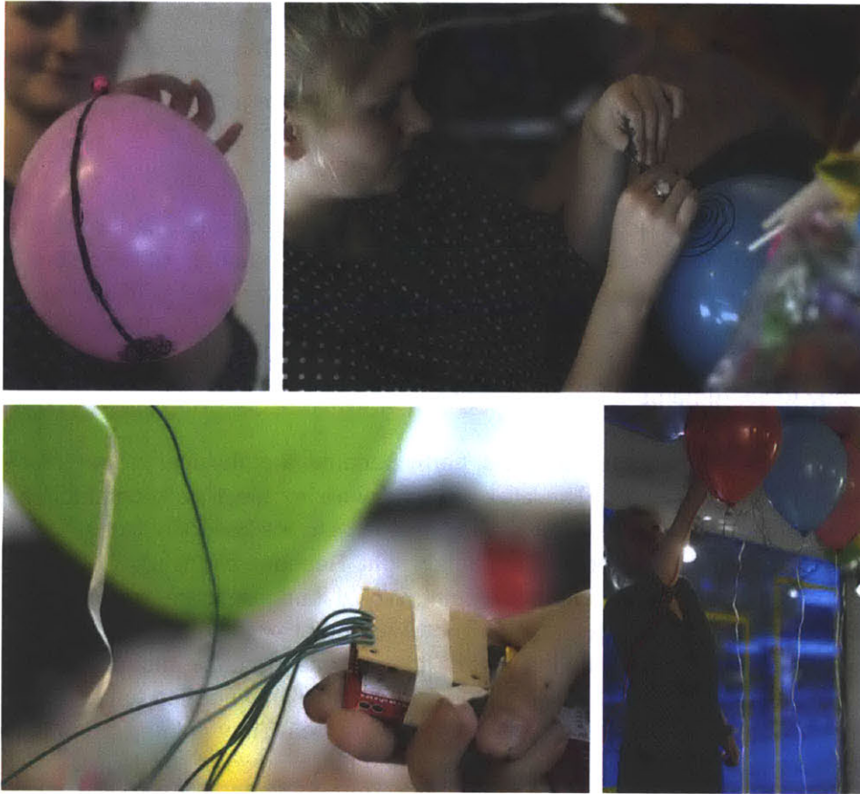
Figure 27: Building the balloonophone. Top left: Tying conductive thread to a balloon with a line of conductive paint on it. Top right: Painting a spiral of conductive paint. Bottom left: a connector to hold wires in place. Bottom Right: installing the balloonophone.
