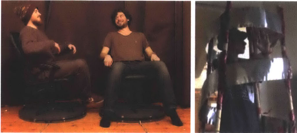
Figure 11: Invented furniture-scale instruments. Left: Musical chairs that trigger different sounds depending which direction they tilt. Right: A spiral instrument that surrounds the body with contacts to mute and unmute music tracks.
