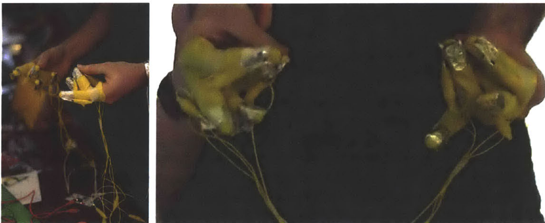
Figure 23: The musical gloves. The body is grounded, so the thumbs can be used to trigger any of eight notes by touching the foil on the fingers. In the image on the right, he is playing a C major chord (C and E the left hand, G and high C on the right hand).
