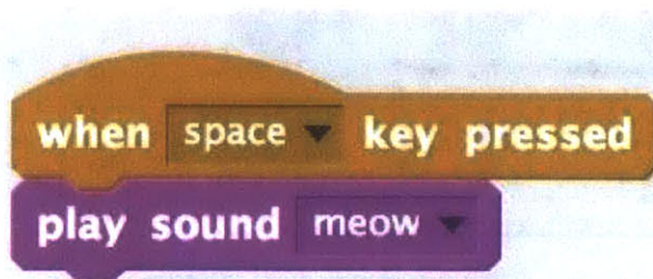
Figure 13: A complete Scratch program for MaKey MaKey. It triggers a meow sound when you press the space key.
