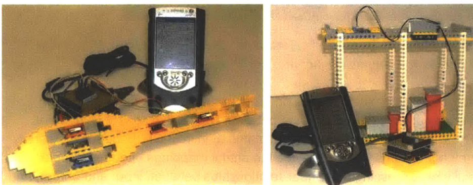
Figure 14: MICK musical instrument construction kit. Left: a guitar with switches. Right: a sliding car with a light sensor.
