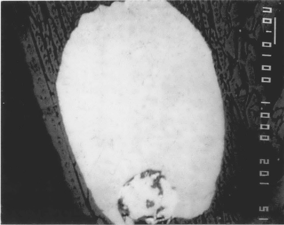
Figure 32. DH 2.1-1: SEM image of copper prill and matte.
