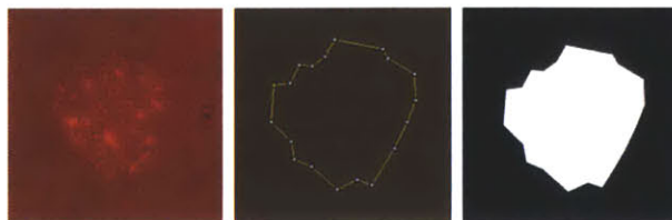
Figure A.4 – Re-scaled fluorescence image of a decomposed triangle-shaped particle (left), its corresponding bright-field image (center), from which a particle mask (right) can be extracted using the freehand selection tool.
