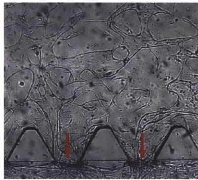
Figure 3.6 – A representative bright-field image showing a portion of the central vascularized region of the flow device. Red arrows indicate openings where particles can enter the microvascular network (above) from the adjacent medium channel (below).
