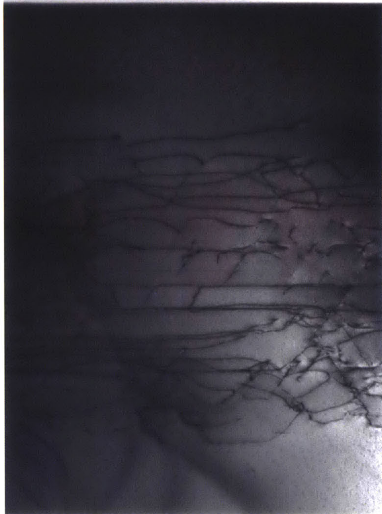
Figure 7: Typical cross section TEM micrograph of a linearly graded \text{InAs}_x\text{P}_{1-x} buffer imaged with the 220 two-beam diffraction condition. The thin dark lines running nearly horizontal are misfit dislocations. No threading dislocations are observed in the cap layer. The image was edited with non-linear brightness and contrast layers in addition to sharpening effects to enhance the visibility of the dislocations.
