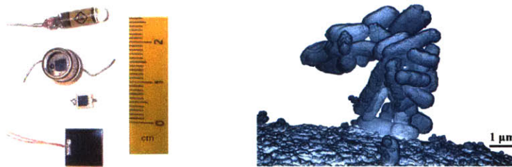
Figure 2. Left: Silicon and Germanium photodiodes ; Right: E. Coli viewed at 10,000x from an electron microscope. Both images are re-used via Creative Commons.
