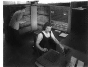
FIGURE 4: MAN AND WOMAN WORKING WITH IBM TYPE 704 ELECTRONIC DATA PROCESSING MACHINE USED FOR MAKING COMPUTATIONS FOR AERONAUTICAL RESEARCH. NASA
