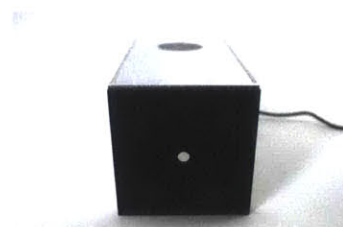
FIGURE 42: INSTRUMENT TYPE SLR2 650NM BANDPASS FILTER APERTURE
