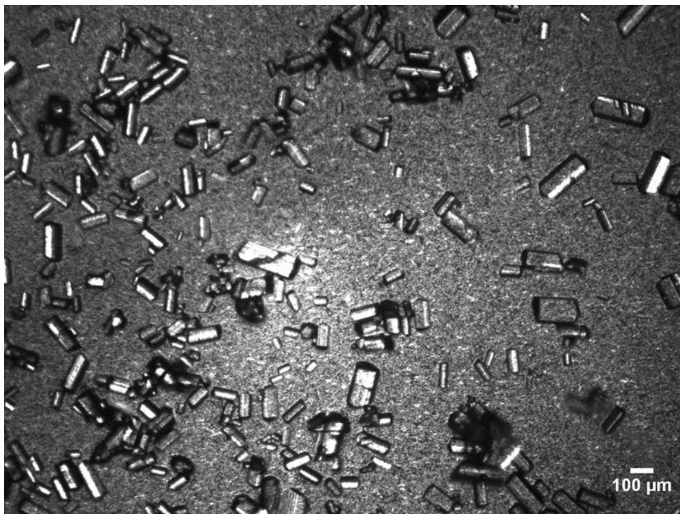
Figure 4.11. Microscopy image (with polarizers) of LAM product crystals at the end of concentration control after continuous DIJ seeding (scale bar = 100 \mu\text{m} ).
