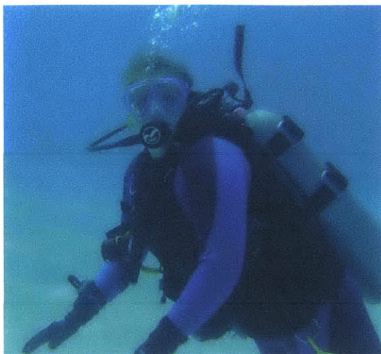
Figure 1-1: Open circuit scuba system: the diver inhales air from the tanks and exhales it to the surrounding environment [3]
