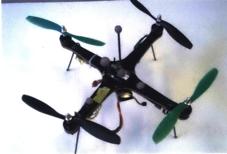
Figure 5-1: The BuddyQuad, a Quadrotor Designed at the Aerospace Controls Lab
