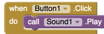
Figure 2. The simplest app behavior requires at least two blocks: An event handler and a resulting action. Here, a sound is played when a button is pressed.
