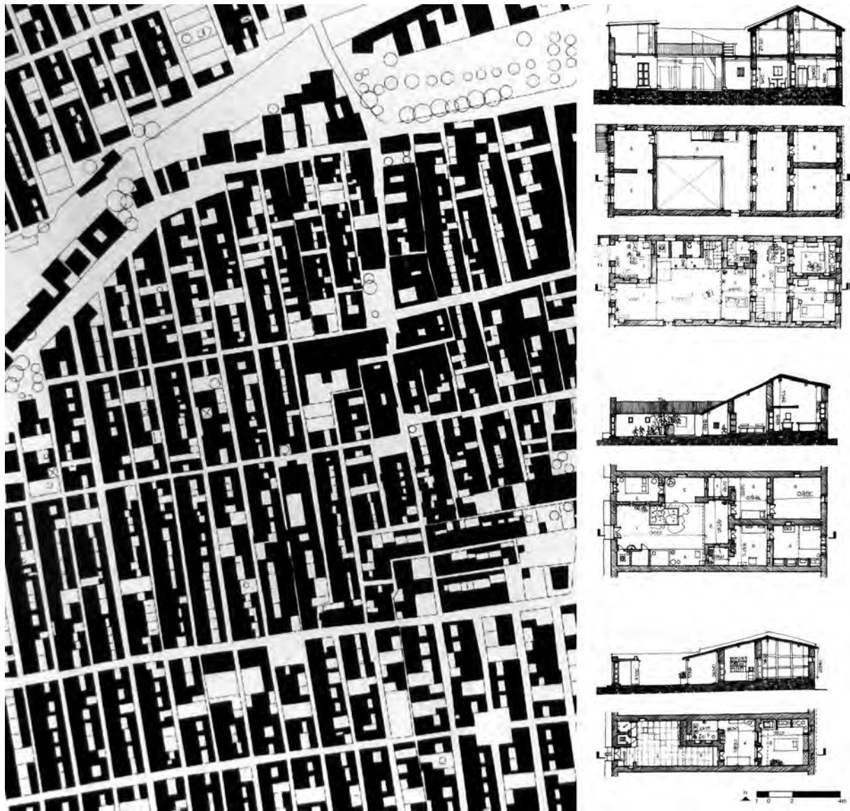
Figure 2.3 – Mistri Madhapar neighborhood site plan (left) and three variations of the house typology (right). Drawings by Shilpa Mevada (Mevada, 2008, p. 26, 52, 58, 62)
