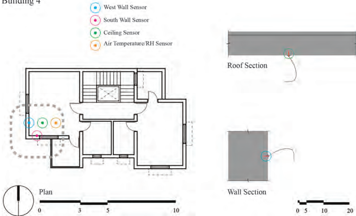
(a) Plan and Wall and Roof Sections Showing Sensor Locations in Building 4.
