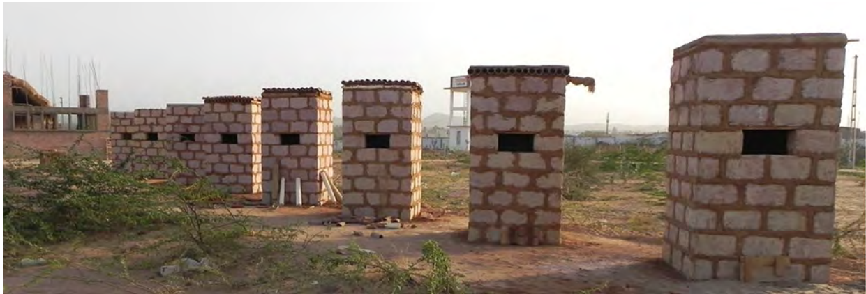
Figure 1.7 – Bhuj Test Chambers with Thermally Massive Roof Assemblies. (Satrasala, 2014, p. 43)
