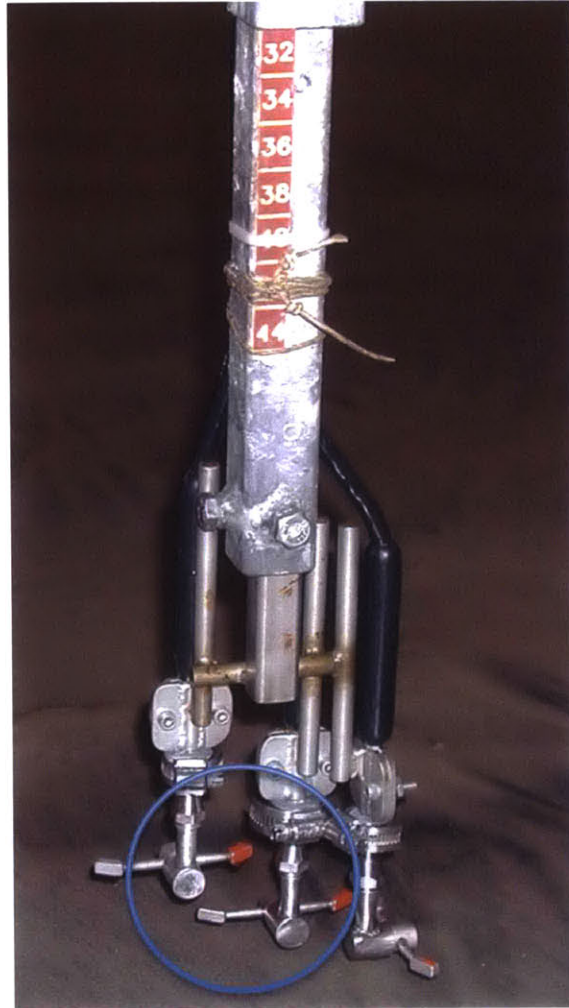
Figure 4: Close up on one instrument: an acoustic doppler velocimeter
