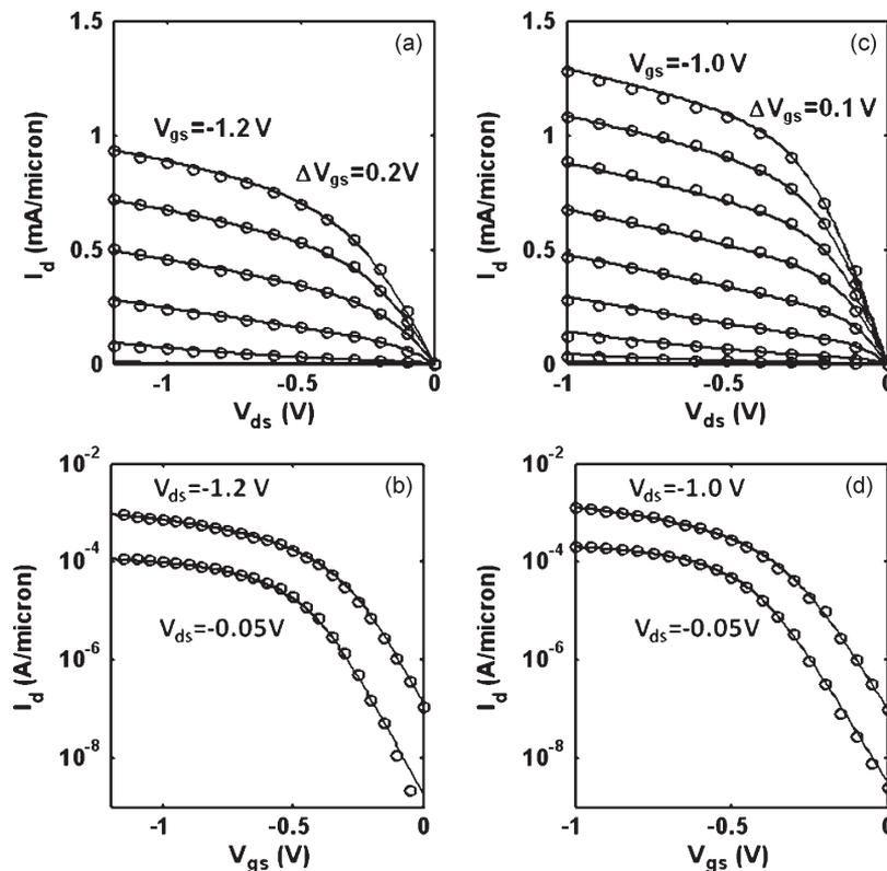
Fig. 5. Comparison of model current (lines) with data (circles). (a) and (b) For a 65-nm technology uniaxially strained pFET technology with poly-SiON gate stack [13] and gate length  $L_g = 35$  nm. (c) and (d) For a 32-nm technology uniaxially strained pFET with a metal-gate high- $k$  stack [Intel IeDM 08] and gate length  $L_g = 32$  nm. Device parameters are given in Table I.
