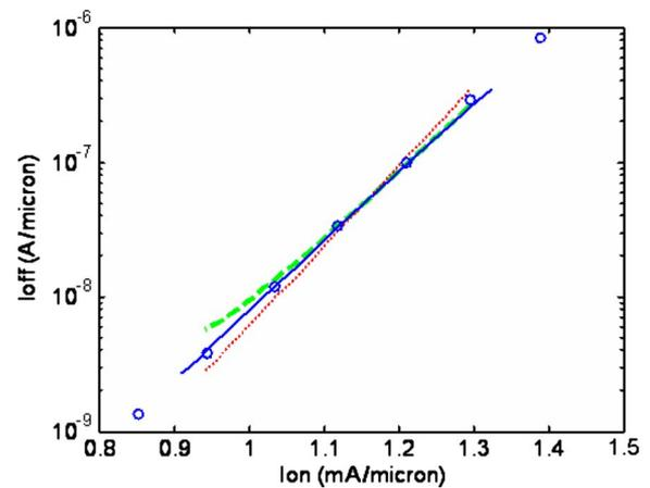
Fig. 6. Modeled versus measured  $I_{off}(V_{GS} = 0 \text{ V}, V_{DS} = 1.2 \text{ V})$  versus  $I_{on}(V_{GS} = 1.2 \text{ V}, V_{DS} = 1.2 \text{ V})$  for the nFET technology in Fig. 3. Data from [13] are depicted by points. For details of the model-calculated lines, refer to the text.
