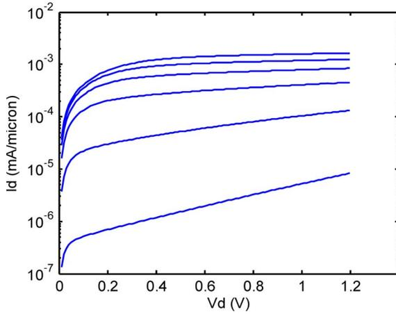
Fig. 3. Model output characteristics as in Fig. 4(a) in a semilog plot to illustrate the continuity of the model from weak to strong inversion and from linear to saturation regions.
