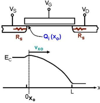
Fig. 1. Virtual source point  $x_o$  in the channel of a modern short-channel MOSFET. The carrier charge and velocity, used in (1) and through this work, are defined at this point (at the peak of the conduction band profile).
