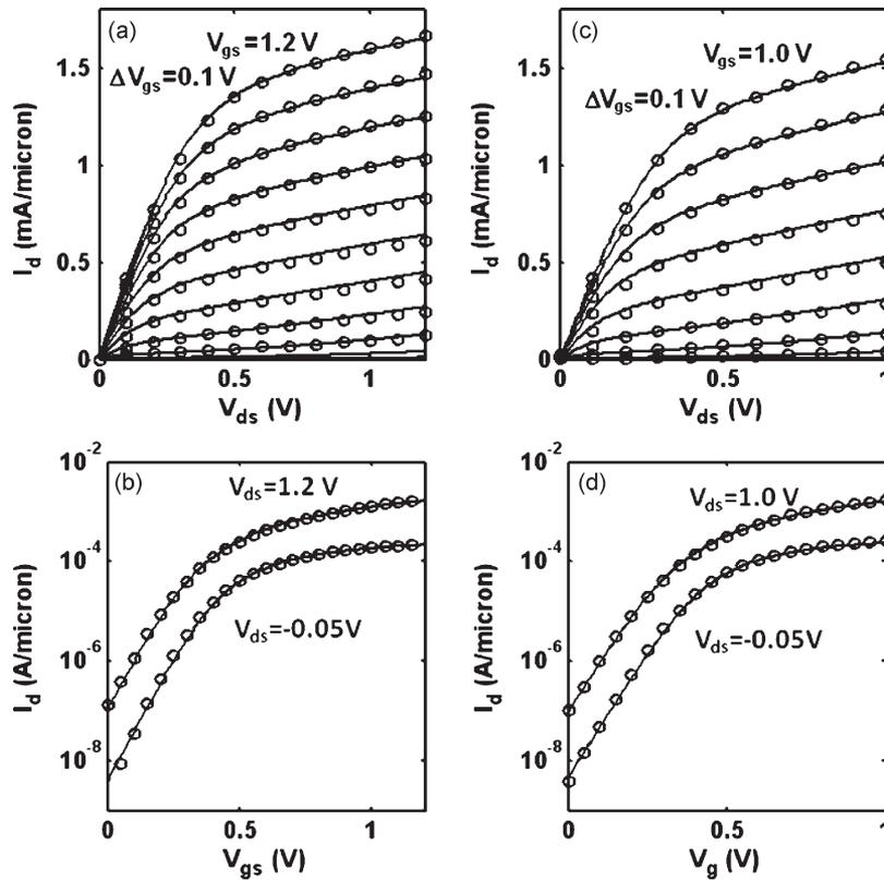
Fig. 4. Comparison of model current (lines) with data (circles). (a) and (b) For a 65-nm technology uniaxially strained nFET technology with poly-SiON gate stack [13] and gate length  $L_G = 35$  nm. (c) and (d) For a 32-nm technology uniaxially strained nFET with a metal-gate high- $k$  stack [14] and gate length  $L_G = 32$  nm. Device parameters are given in Table I.
