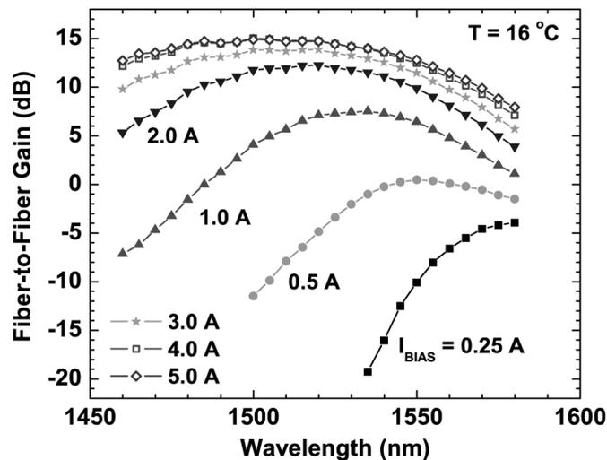
Fig. 2. Small-signal gain spectra of the packaged SCOWA for several bias currents. Baseplate temperature =  $16^\circ\text{C}$ .
