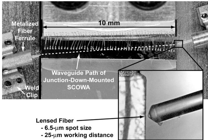
Fig. 1. Top-down photograph of junction-down-mounted SCOWA packaged using lensed-fiber pigtailed. SCOWA length = 10 mm. SCOWA facet angle =  $5^\circ$ . SCOWA soldered to Cu-W submount. Lensed-fiber parameters: fiber = SMF-28, spot size =  $6.5 \mu\text{m}$ , working distance =  $25 \mu\text{m}$ .
