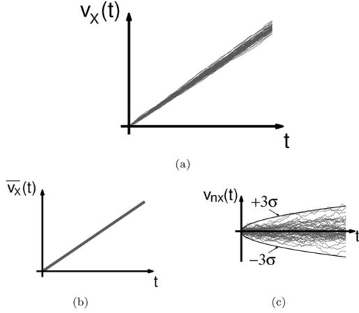
Fig. 3. In transient noise analysis, it is ensemble averages and not time averages that are most important. (a) Ramp voltage plus random walk noise. (b) Average ramp voltage. (c) Random walk noise voltage showing  $3\sigma$  bounds.
