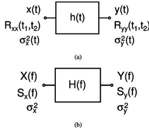
Fig. 1. Overview of time domain and frequency domain analyses. (a) Time domain noise analysis input and output variables. (b) Frequency domain noise analysis input and output variables.
