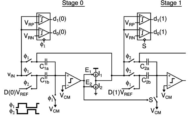
Fig. 9. First two stages of pipeline ADC. Note that the first-stage sampling and bit-decision clocking are controlled by the system clock, but for the second and subsequent stages, the sampling and bit-decision clocking are controlled by the comparator of the previous stage.
