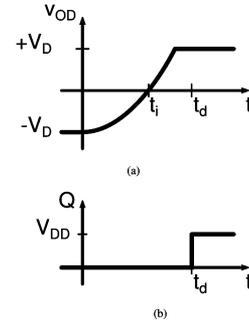
Fig. 12. Ideal timing for comparator with preamplifier. The preamplifier output voltage is clamped at  $\pm V_D$ . (a) Preamplifier output voltage showing the response time  $t_i$  that it takes for the preamplifier output to reach the comparator threshold. (b) Output logic signal changes state after total comparator delay  $t_d$ .
