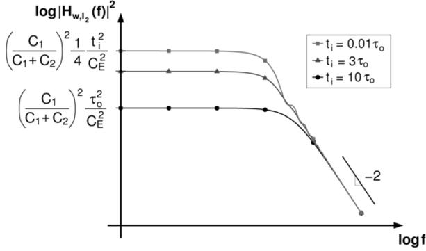
Fig. 16. Charging current transfer function  $H_{w,I_2}(f)$  during preamplifier response time for different preamplifier output resistances causing variation in  $t_i$  relative to  $\tau_o/2$ . A broadband preamplifier ( $t_i \gg \tau_o/2$ ) results in more noise cancellation and lower transfer function gain.
