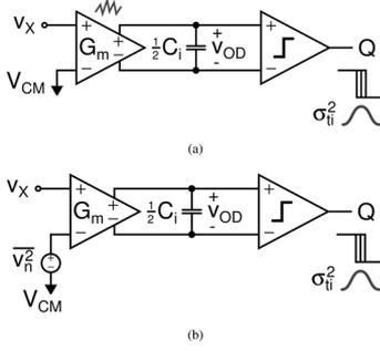
Fig. 5. Input-referred noise modeling. (a) Noisy preamplifier results in threshold comparator jitter at output threshold crossing. (b) Noiseless preamplifier with input-referred noise voltage ( $v_n^2$  in  $V^2$ ) results in the same jitter at the input threshold crossing.
