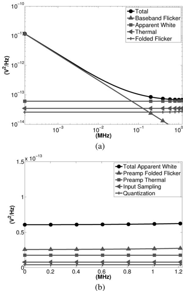
Fig. 19. Theoretical breakdown of PSD noise for  $f_s = 2.4576$  MHz. (a) Theoretical breakdown of aliased components. (b) Theoretical breakdown of apparent white noise sources.
