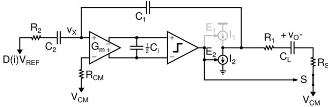
Fig. 17. Noise contribution from sampling and configuration switches.
