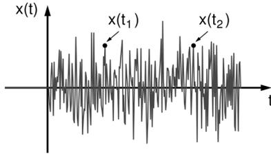
Fig. 2. Step noise signal  $x(t)$ . Underlying WSS noise process  $\nu(t)$  applied at  $t = 0$ . If  $t_1$  or  $t_2$  is less than zero, the autocorrelation for  $x(t)$  is zero, and if  $t_1$  and  $t_2$  is greater than zero, the underlying WSS autocorrelation  $R_{\nu\nu}(t_1, t_2)$  defines the autocorrelation of  $x(t)$ .
