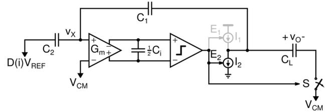
Fig. 14. Noise contribution from fine-phase charging current  $I_2$ .
