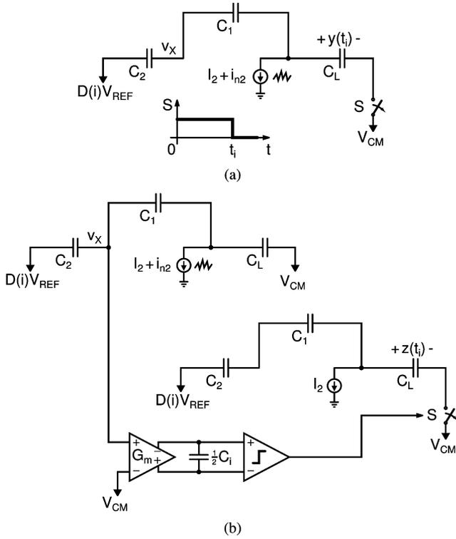
Fig. 15. Charging current noise analysis with correlated sampling jitter. (a) Open-loop random walk noise voltage  $y(t_i)$  on  $C_L$  after response time  $t_i$ . (b) Noise voltage  $z(t_i)$  sampled on  $C_L$  due to jitter in comparator decision only.
